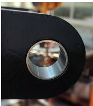
LOW MAINTENANCE BUSHES AND CHROMIUM PLATED PINS.
