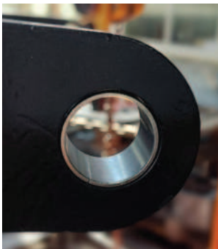
LOW MAINTENANCE BUSHES AND CHROMIUM PLATED PINS.
