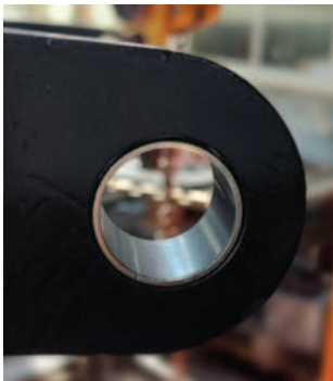
LOW MAINTENANCE BUSHES AND CHROMIUM PLATED PINS.
