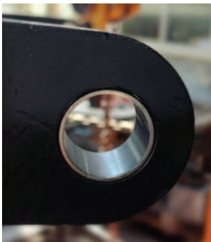
LOW MAINTENANCE BUSHES AND CHROMIUM PLATED PINS.
